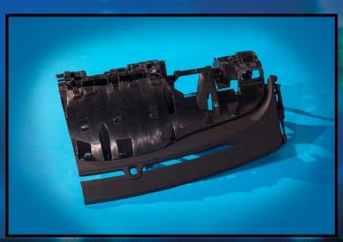
This is the first instrument panel with long glass fiber on a visual surface. An integration of the polished area and grained area to one part in one tool contributed to the development of this innovation. Reducing the area of the soft skin and avoiding additional tooling for the partial visual structure of the long glass fiber material was a cost savings factor. This new design contributed to a 300g weight reduction and a \$2.2 per vehicle cost savings.
