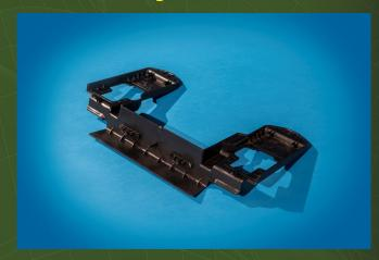
Metal clips and springs were eliminated by designing an in-molded W shaped plastic clip with a 4-way locator providing efficient attachment per requirements and eliminating additional costs for fasteners and assembly. The plastic part comes out of the tool with the clips molded in. The patented winged spring clip design locates, locks and retains in a single snapping action. A cost save of \$0.17 per clip/\$2.19 per vehicle resulting in \$250K per year; and a 10% weight saving is achieved.
