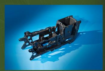
This floor console carrier is unique with its 2.0 mm nominal thin wall thickness (with ability to implement lightening holes) and 40% Long Glass Fiber PP construction with first surface quality appearance. A 30% mass savings resulting in a 2.2 lb/.99 kg weight savings, and a 15% cost savings was achieved. Lateral stiffness targets were exceeded eliminating the need for metal brackets (\$1.50). It is also the first time injection molding was used to process this type of a component.
